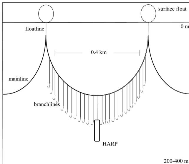
Fig. 1. Schematic of longline fishing set with HARP attached.
