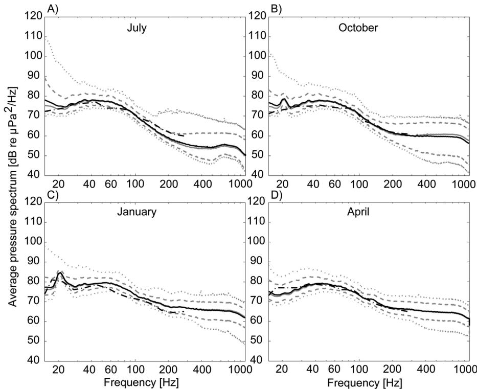
FIG. 3. Representative monthly sound pressure spectrum levels from 15 to 1000 Hz for (A) July (summer), (B) October (fall), (C) January (winter), and (D) April (spring). Solid black line is the 2013–2014 monthly mean and dash-dotted black line is the 1966 monthly mean for given month. Solid grey line is the median, dotted grey lines are 10th and 90th percentiles, and broken grey lines are 1st and 99th percentiles.
