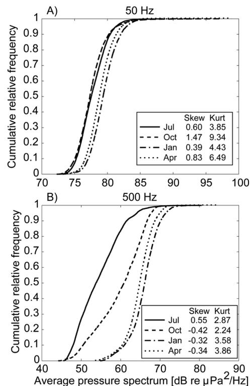
FIG. 4. Cumulative density functions of average sound pressure spectrum levels at (A) 50 Hz and (B) 500 Hz during four representative months. The skewness and kurtosis for each presented month are in the inset.
