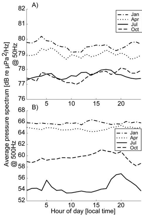
FIG. 5. Examples of hourly average sound pressure spectrum levels at (A) 50 Hz and (B) 500 Hz during four representative months from June 2013 to May 2014.
