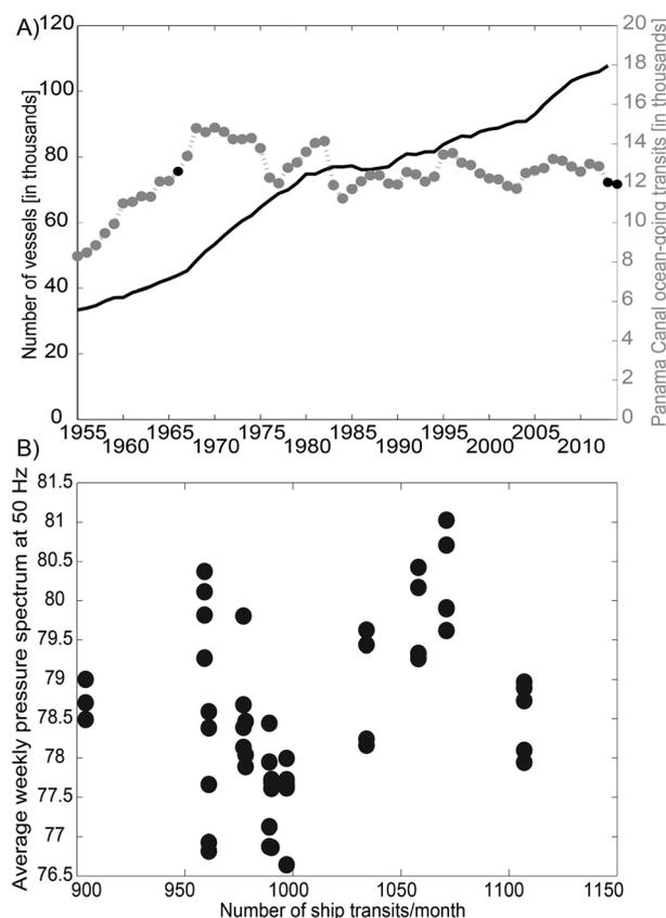
FIG. 2. (A) Shipping trends since 1955 as total number of vessels (black solid line) and total annual number of ocean-going ship passages through the Panama Canal (light grey dots; with 1965, 2013, and 2014 data highlighted as black dots). (B) Number of monthly ship transits through the Panama Canal compared to the average weekly pressure spectrum levels at 50 Hz.
