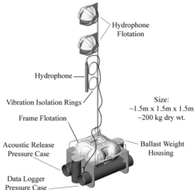
**Figure 2.** Photograph of an ARP ready for deployment. The hydrophone electrical cable and hydrophone are attached along a polypropylene line between the instrument package and the two hardhat glass spheres.
