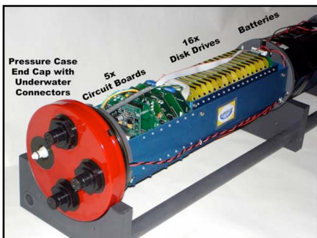
Fig. 1. HARP data logger mounted on aluminum pressure case end cap (7" diameter x 2" thick) with underwater connectors. The data logger consists of a backplane populated with five primary printed circuit boards (clock, A/D, CPU, RAM, Ethernet/IDE controller), a disk block with 16 laptop computer disk drives and 48 D cell alkaline batteries. Another pressure case filled with alkaline batteries can be included for long-term deployments.
