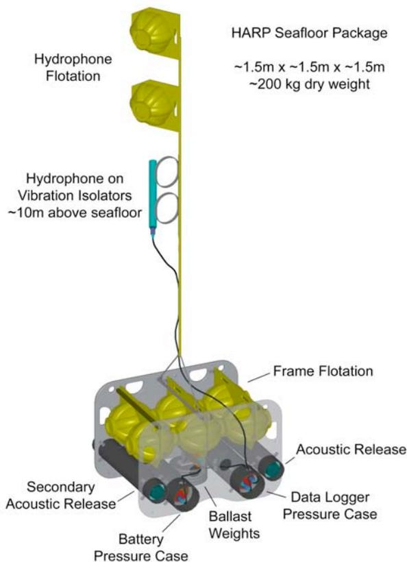
Fig. 3. HARP Seafloor package including data logger and acoustic release electronics pressure cases, ballast weights, glass flotation sphere in yellow hard hats, and hydrophone tethered ~ 10m above seafloor.
